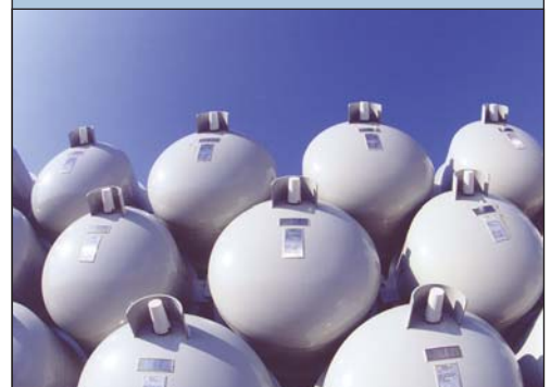
A crane operator (above) unloads a cylinder filled with uranium hexafluoride at the Paducah plant. This stack of new cylinders (below) will eventually be filled with depleted uranium, a by-product of enrichment.
