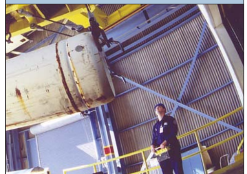
A crane operator (above) unloads a cylinder filled with uranium hexafluoride at the Paducah plant. This stack of new cylinders (below) will eventually be filled with depleted uranium, a by-product of enrichment.
